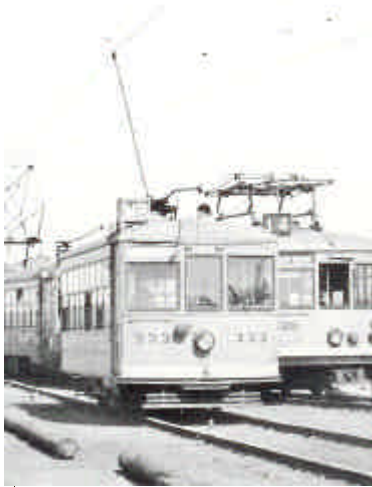
Birney Car 333 shuttled passengers to Mission Beach from the Ocean Beach line in 1924. SDERy bought 35 of the one-man single truck "Cooties" to lower costs on the Point Loma Railroad routes. [Photo from R. V. Dodge, Rails of the Silver Gate ]
